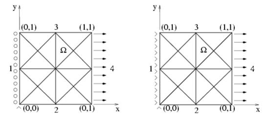
Figure 3: Geometry and coarse mesh  $\mathcal{T}_0$  of 1D beam (left) and 2D beam (right).
