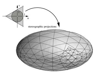
Figure 3: Covering the ellipsoid with triangular patches.
